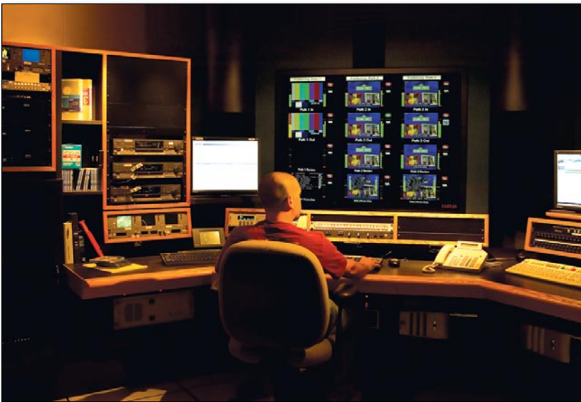
PBS editor Robert Sottile streams three channels and takes an IMX50 50MB file and rerecords it to an 8MB file in the flattening room.
